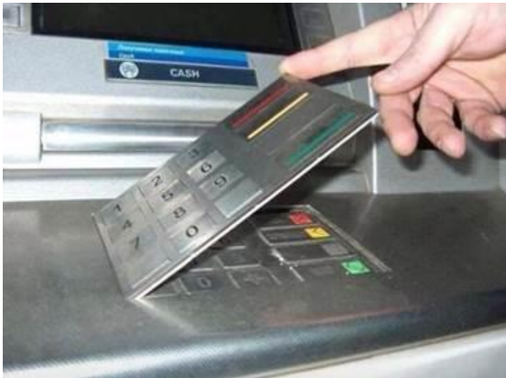
Example of a keyboard overlay designed to steal debit card PIN Numbers.
